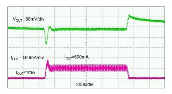
$\label{eq:classical} XCL241 $$V_{IN}=5.5V,\,V_{OUT}=3.6V,\,I_{OUT}=1mA\Leftrightarrow 500mA(tr,tf=1us),\,Ta=25\%$
