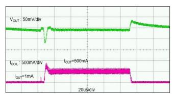
$\label{eq:cl241} XCL241$   $V_{IN}\text{=}3.8V,\,V_{OUT}\text{=}1.8V,\,I_{OUT}\text{=}1\text{mA} \Leftrightarrow 500\text{mA(tr,tf=1us)},\,Ta\text{=}25^{\circ}\!C$
