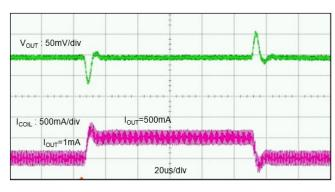
$\label{eq:cl242} XCL242 $$V_{IN}=3.8V,\ V_{OUT}=1.8V,\ I_{OUT}=1mA\Leftrightarrow 500mA(tr,tf=1us),\ Ta=25^{\circ}C$
